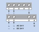
The actuator M9304-GGA-1N can also be controlled using the Positioner (M9000-PA and M9000-PF) with a control signal of DC 0...10V.
