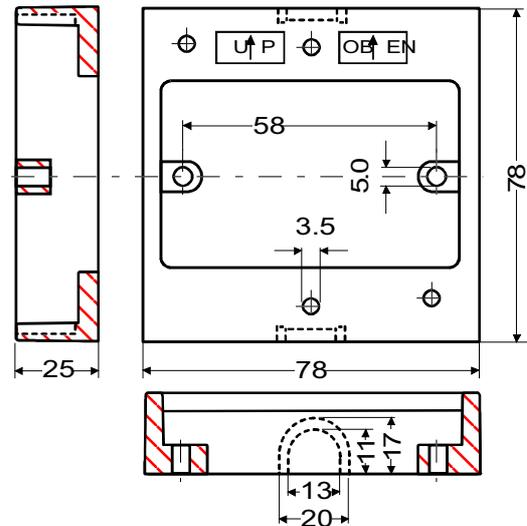
Figure 2: TM-1100-8931 Surface Mounting Kit
