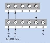
The actuator can also be controlled using the Johnson Positioner (PA-PF) with Control signal of DC 0...10 V. For further information concerning the PA and PF Positioner please refer to data sheet 6.20.
