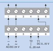
For parallel operation of the actuators, the DC 0...10 V output signal U = DC 0...10 V is connected, from the master actuator trough terminal 6, to the slave actuator trough terminal 5 etc.
