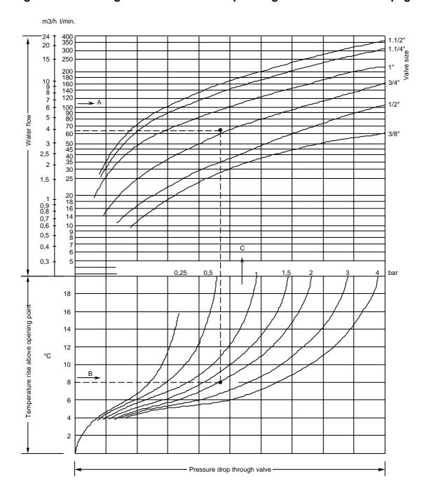
Note: 1 dm<sup>3</sup>/s = 3.6 m<sup>3</sup>/h = 15.8 U.S. gal./min. = 13.2 U.K. gal./min. 1 bar = 100 kPa = 0.1 MPa  $\approx$  1.02 kp/cm<sup>2</sup> = 1.02 at  $\approx$  14.5 psi.
